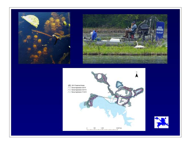
The application method uses computer controlled equipement mounted on an airboat, that delivers the appropriate dosage based on the speed and location of the boat, as determined by a GPS link. Our consultant performed a total of three applications between early May and July. The map shows the airboar tracks on each of the applications.
