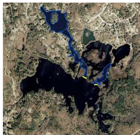
2007: The 2007 treatment area (in blue) totaled 18 acres. Water-impermeable barriers (in yellow) kept the Sonar from dissipating in the Main Pond.
